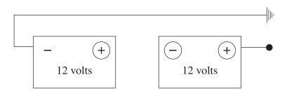
(e) In the diagram below, draw lines to show how to connect the terminals to maintain battery output voltage at 12 volts.
